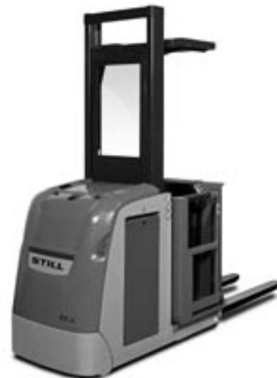
EK-X single lift mast height 2,000/2,500 mm
